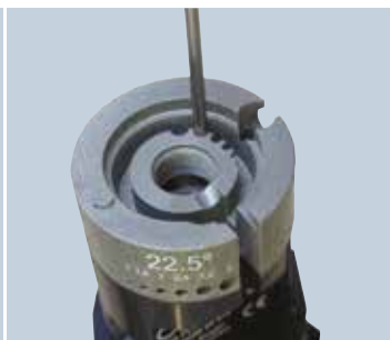
Squaring an electrode tip
