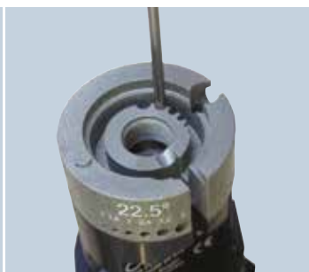
Squaring an electrode tip
